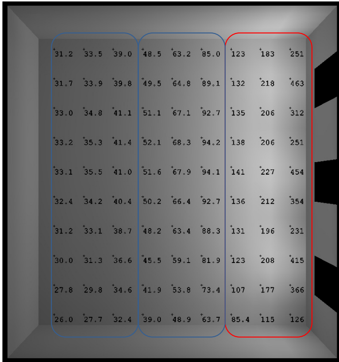
Figure 10.10.4 – AGi32 Illuminance Levels at 1 PM on September 22, 2009
